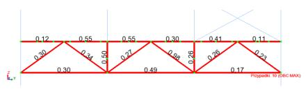
Fig. 5. Stress-strain state of lattice in axis "3" following strengthening
